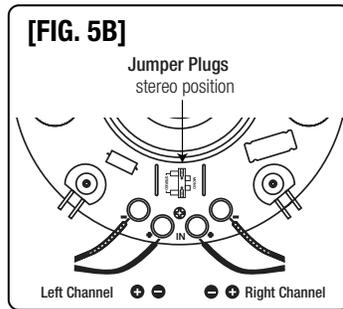
**STEREO POINT SOURCE FIG. 5B**-8 ohms: Use this configuration to combine left AND right channels for full fidelity sound from a single loud-speaker stereo source. Set jumper plugs in the stereo position. Connect right and left signal wires to the spring-loaded terminals on the rear of the speaker.
