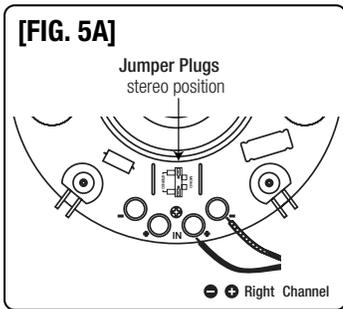
**STEREO FIG. 5A**-8 ohms: Use this configuration to drive one channel (left OR right) of a stereo pair. Set jumper plugs in the stereo position. Connect the right or left signal wire to the right set of terminals on the rear of the speaker.
