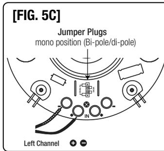
**MONO/STEREO FIG. 5C**-4 ohms: Use this configuration to drive one channel (left OR right) of a stereo pair with a 4 ohm speaker load. Set jumper plugs in the mono position. Connect the right or left signal wire to the left set of posts on the rear of the speaker. Acoustic output of the speaker is increased by 3 dB in this configuration.
