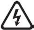
The lightning flash with arrowhead symbol, within an equilateral triangle, is intended to alert you to the presence of un-insulated "dangerous voltage" within the product's enclosure that may be of sufficient magnitude to constitute a risk of electric shock to persons.
