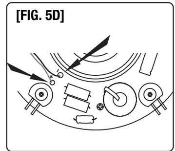
**BIPOLE/DIPOLE FIG. 5D**-4 ohms: Use this configuration for home theater surround applications. For bipole mode, connect as in the Mono/Stereo instructions (FIG.5C): one speaker to each surround channel. For dipole mode, connect speaker inputs the same as Mono/Stereo instructions (FIG.5C), but reverse the + and - connections of the red and black tweeter wires to put one of the tweeters out of phase.
