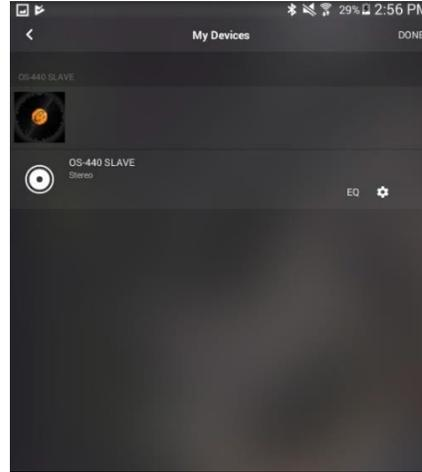
3. At the bottom of the Device Settings page, press the 'DDMS SETTING' button and then press the 'PAIR' button. After a moment, the Slave OS-440 amplifier's WiFi LED will blink green. This means the Slave OS-440 amp is ready. Repeat for additional OS-440 slave amplifiers (up to 8).
